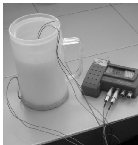
Figure 15. Plastic double-wall glass and the measurement system.
